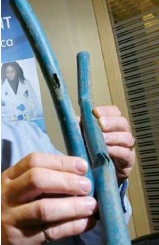
Figure 1: Deteriorated pieces of polybutylene pipe
