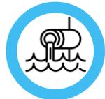
**Outfall:** Discharge point by which stormwater leaves the pipe system and enters the water system (i.e. lake, creek, river).
