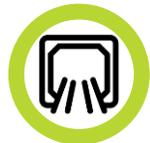
**Culvert:** A relatively short segment of pipe that is typically used to transport water underneath a roadway or other type of earthen embankment.
